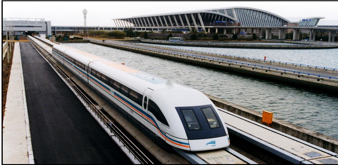
Figure 4.2.1. The Transrapid Shanghai Maglev Train, with a top speed of 431 km/h (268 mph). It is the first and only commercial high-speed maglev line in the world.
